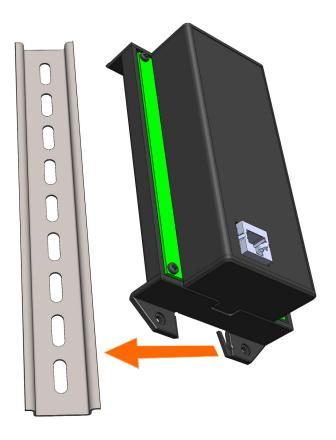
Figure 3 - 1516LI Mounting on the DIN Rail Example
