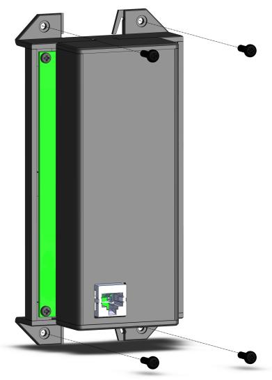
Figure 2 - Wall Mounting with Screws
