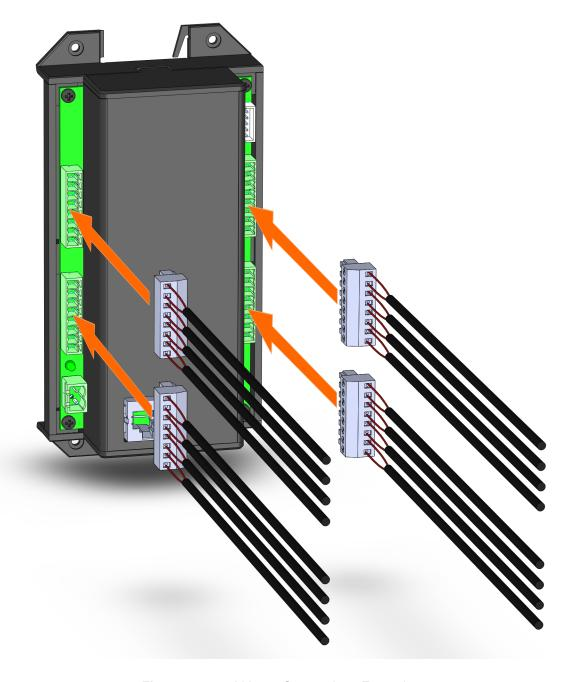
Figure 9 - 1516LI Input Connections Example
