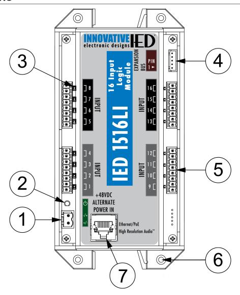
Figure 1 - Front View - 1516LI Connections
