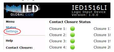
Before accessing the Settings page, one must enter the current password in the edit box shown below. By default from the factory, the password is "iednet" (without the quotes). This password can be changed on the Settings page, once accessed.
