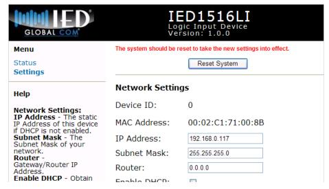
GLOBALCOM®/GCK Note: If the GLOBALCOM® or GCK system this device is being added to is itself on a compatible 10.x.y.z network, it should not be necessary to access the web pages at all. Instead, System Management Center (SMC) will discover the 1516LI device and set it up for expansion and any new IP address as defined in the project file.
