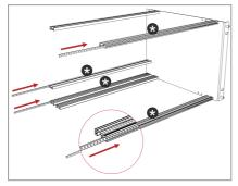
4. Use the remaining 12 M4 screws to connect the other side panel to the mounting rails.
