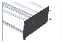
3. Slide an M3 bolt strip into each of the four mounting rails shown here.
