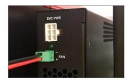
2. Connect the other end of the power cable to the fan cover.
