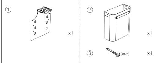
1 Position and mount the holder 1 to the table using all wood screws 3.
