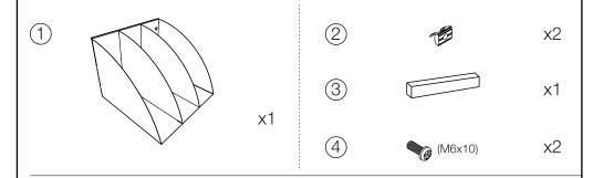
1 Place the sliding nuts2 approximately 240 mm apart. Push them into the lower toolbar T-slot, then turn to make the spring face away from you.
