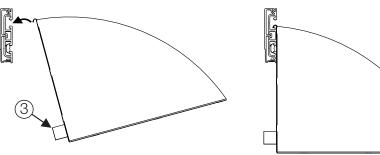
3 Align the screw holes of the sliding nuts② with each respective hole of the shelf①. Once aligned and hooked, mount the screws④.
