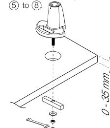
4 Replace clamp bracket with grommet bracket(2) and bolt(3).
