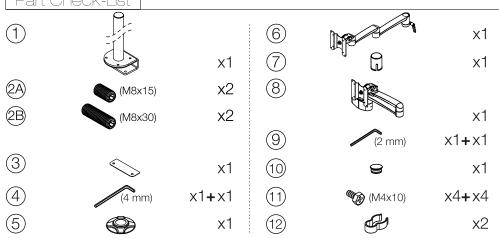
Position and mount the clamp 1 to the table. For tables thinner than 21 mm, use screws 2. Position the metal sheet 3 and fasten it using the screws and Allen key 4 (See illustration).
