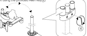
Insert the prepared monitor arm from step 2. Then, attach the plastic cover to cover the cavity. Once all pieces are set in place, tighten all four small screws using the small Allen key 7. To make all joints and arms completely rigid, use Allen key 4.
