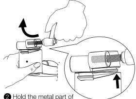
Hold the metal part of the arm with a firm grip. Use leverage to bend the lever upwards with as much force as possible. The bottom of the clamp will surface as seen in the zoomed-in illustration.
