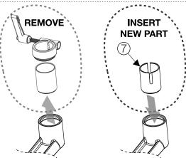
4 Remove the black plastic clamp and replace the old bushing with the one provided in the carton box 7.
