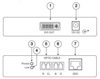
Figure 2: 621R DVI Optical Receiver
