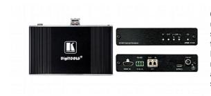
676R is a high-performance HDMI fiber receiver for ultra-reach extension of 4K@60Hz (4:4:4) HDMI signals. 676R receives the transmitted optical signal from a compatible transmitter and converts it to an HDMI and RS-232 signals. 676R includes a multi-mode SFP+ transceiver, but can be used with any Kramer certified SFP+ transceiver, such as a single-mode SFP+ transceiver
