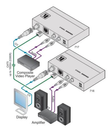
Figure 4: Connecting the Video-Audio Line Transmitter/Receiver System
