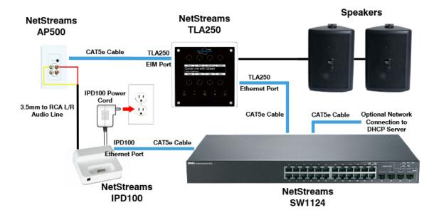
> NOTE: CAT5e cable run between the NetStreams AP500 and the EIM Port on the host device (NetStreams TLA250 in above diagram) should not exceed 60' in length.
