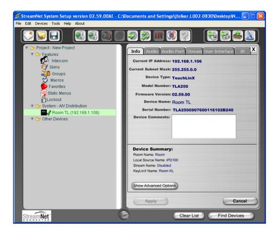
3. On the Device Panel, click on the *Enable Static IP* and enter the IP, Subnet Mask and Gateway addresses of the interface device (TLA250 as shown in the Basic Connection diagram). Optionally, check the *Enable DHCP* checkbox if a DHCP server is to be used. If the DHCP is enabled and a DHCP server are not available, the TLA250 or the SL251 will revert to the Auto IP address settings in the Dealer Setup.
