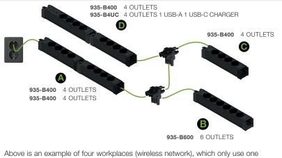
power connection from the property. In order not to overload the first connection in the chain is important that the total power consumption does not exceed 3500W.
