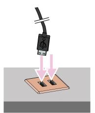
CONNECT AND PLUG IN Connect USB Micro cable to the grommet and to adapter. Lastly, plug it to a wall socket or powerstrip of your choice.
