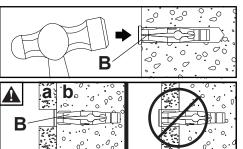
ENG Insert anchor thru drywall (a) flush to concrete (b)
