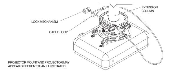
Insert key into lock mechanism and set to open position by pushing in key and rotating until hooks are in open position as shown in figure 2.1.
