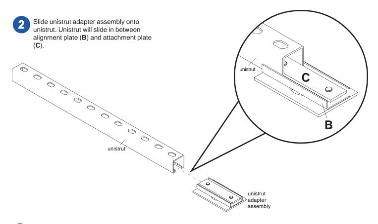
Once unistrut adapter assembly is in desired position, tighten M10 socket head screws (**D**). When attaching the mounting body (**A**) to flush mount tube or extension column. Tighten at least four complete turns ending with one of the small threaded holes aligned with slot in the end of flush mount tube. Insert and tighten one security screw (**E**) shown below right.
