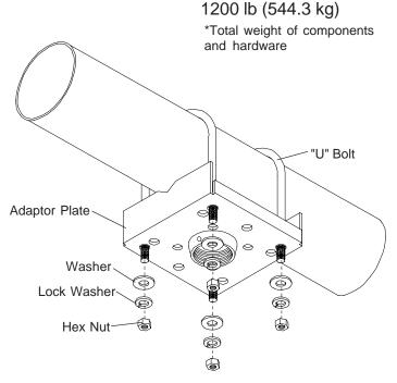
Now tighten Hex Nuts to a maximum of 25 FP (34 NM) so that the lock washer becomes flat. Mount your bracket according to the instructions provided with it.
