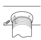
IMPORTANT: Insert the M5 x 10mm screw in the threaded pipe fitting as directed in the extension column instructions. If you are using an extension pipe without a notch, drill a 11/64 (0.172") dia. hole through the pipe and insert the screw through
