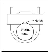
This bracket will only be used on round 2" (max.) pipes to mount extension columns.
