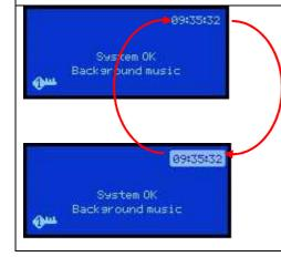
The SYSTEM FAULT signal is achieved with a flashing indication on the frontpanel display. In a normal operating condition, the system time will flash inside a frame. If for any reason the time indicator stops flashing, the unit will be in a SYSTEM FAULT condition. In that case, after 10 seconds, approximately, a watchdog timer will force a reset that will reboot the unit.
