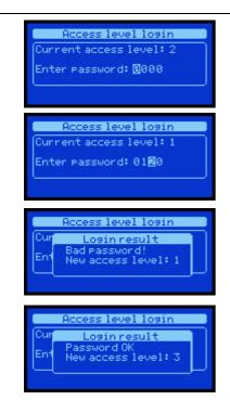
The **ACCESS LEVEL LOGIN** menu allows the user to login and obtain the desired access rights. The system provides three access levels 1-2-3 where level 1 has the lowest priority and level 3 has the highest priority. The screen displays the current access level.
