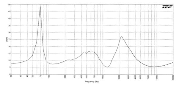
AH94-15-BSG Impedance (ohms) vs. Frequency
