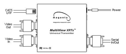
Figure 3-3. Connections on the XRTx 232 Universal Transmitter.
