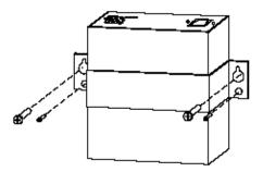
Figure F-1. Receiver Mounting Bracket.
