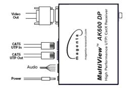
Figure 3-2. Connections on the AK600 for video and audio.
