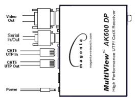
Figure 3-4. Connections on the AK600 232 Receiver
