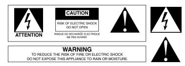
The lightning flash with arrowhead symbol within an equilateral triangle, is intended to alert the user to the presence of uninsulated "dangerous voltage " within the product's enclosure that may be of sufficient magnitude to constitute a risk of electric shock to persons.
