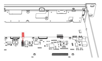
**Step 4:** Remove the 4 screws located around the pin header 'P9' on the main board of the XMP44, and replace them with the supplied M3 spacers as indicated in the image below.
