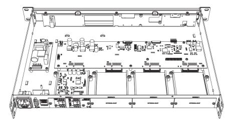
**Step 3:** Remove all the jumpers (6x) on the main board of the XMP44, located besides the USB connector at the center position of the board.
