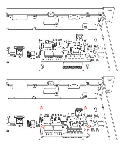
Once inserted and positioned correctly, the ANX44 can be secured to the XMP44 by inserting the 4 original screws (removed in step 3) to the M3 spacers.
