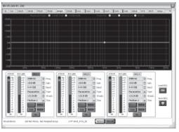
**DEQ:** this is 3-band dynamic equalizer useful to optimize the system's response for different kind of applications and different music genres, or to obtain an optimal behaviour of the system at different levels.
