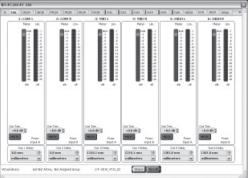
**OUT:** in this page you can see the level of the output signals and the gain reduction if the limiters are activated. You can also trim (±6 dB) the output signals in order to adjust the balance of LF, MF and HF ranges.
