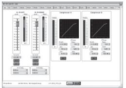
**IN:** In this screen you can adjust the input levels and the input compressors.
