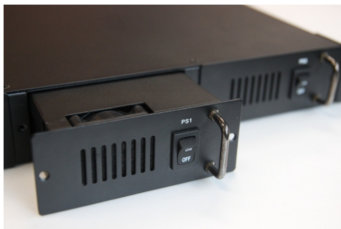
Fig. 8: Hot-swapping of power supplier
