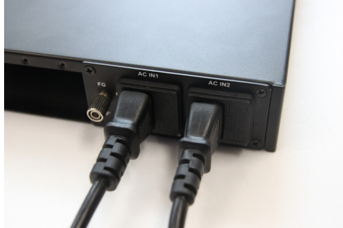
Fig. 6: Connect AC plugs to BR-100
