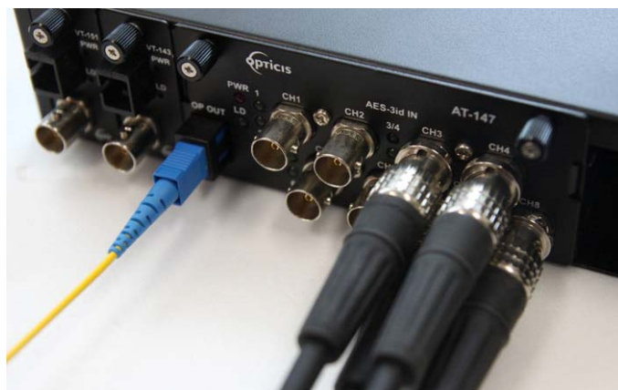
Fig. 15: 4 audio inputs and SC output of AT-1xx
