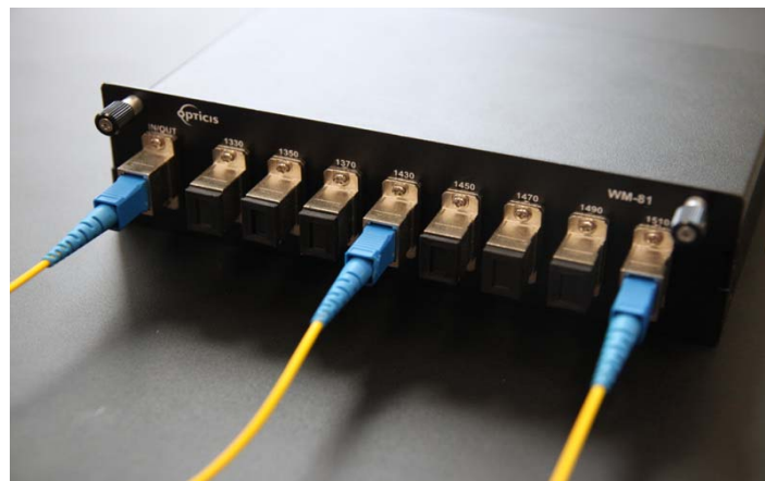
Fig. 13: WM-81 multiplexer to combine optical signal
