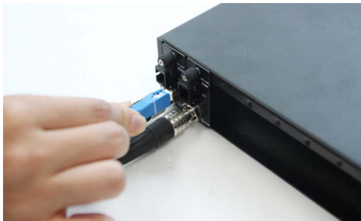
Fig. 11: Plugging SC fiber-optic cable to VT-1xx
