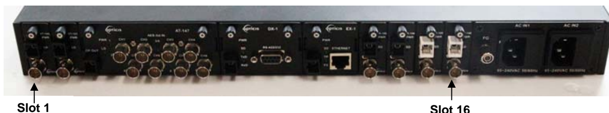
Fig. 9: Slots for extenders on rear side
