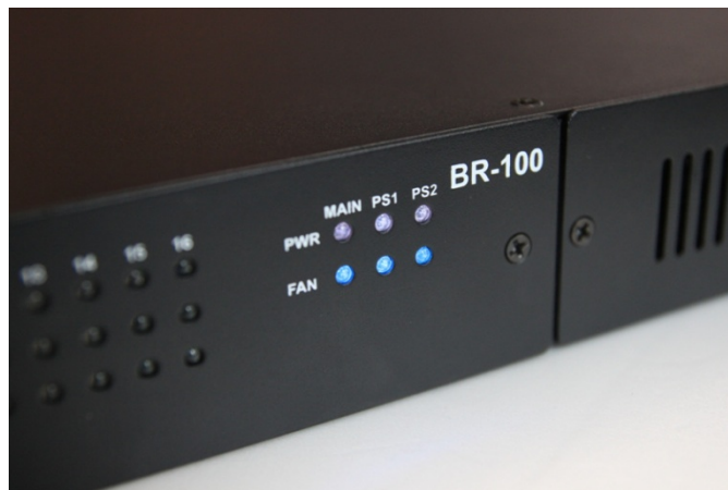
Fig. 7: Frame status LEDs on front panel
