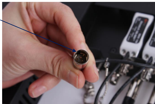
Fig. 10: Insertion guide inside of ITT power connector of SDIX-100
