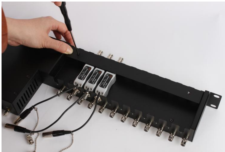
Fig. 6: Fixing of upper cover in BR-300 or BR-310
