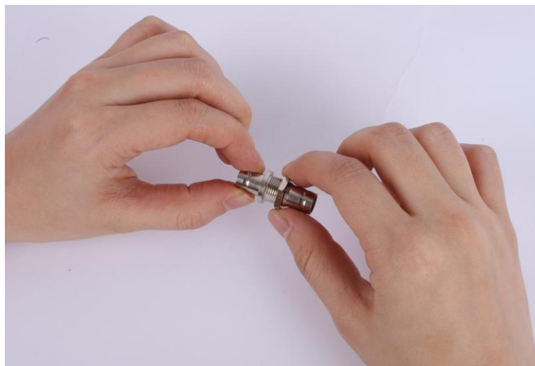
Fig. 2: Screwing larger hexagonal head nut into a 75Ohm BNC bulkhead receptacle
