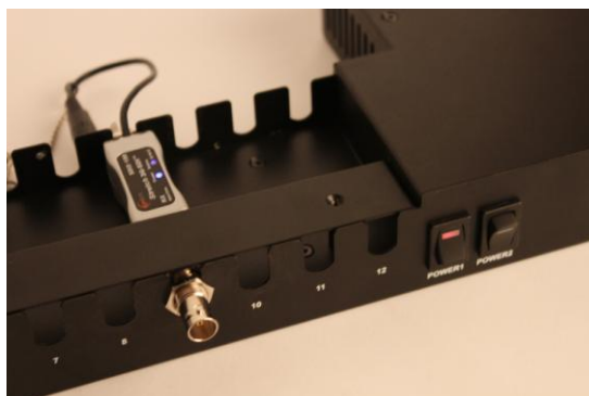
Fig. 13: Normal power status of BR-310 and SDIX-100 (In this case only Power 1 is running)
