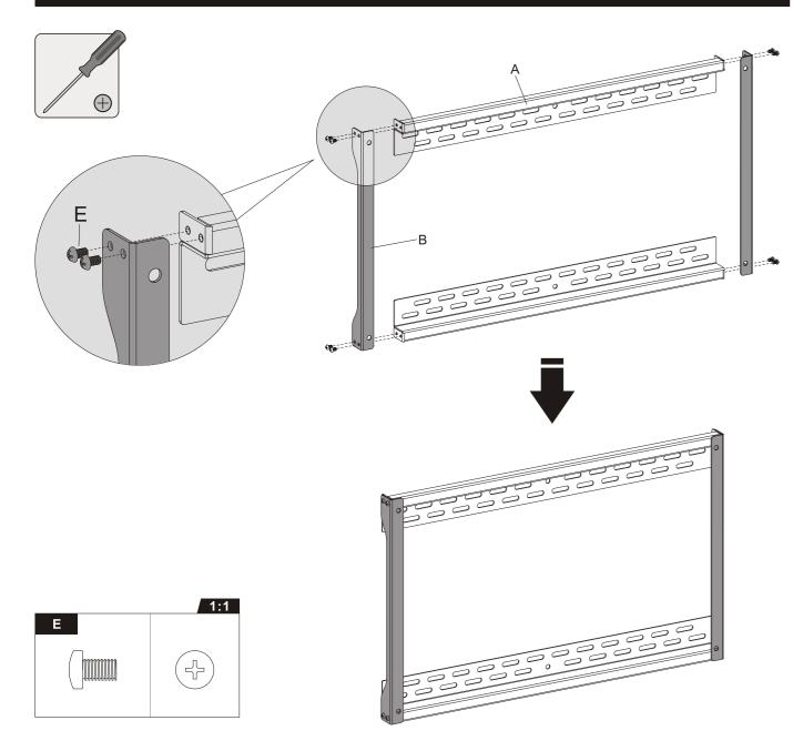
Attach the connecting plates to the wall plates using the appropriate screws.
