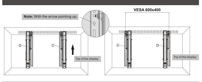
For **VESA 600x400**, the positions of "D" and "C" are exchanged.
