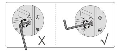
Note: • Don't use the short end of Allen key to tighten the adjustment screw. • Use the long end of Allen key to tighten the adjustment screw.
