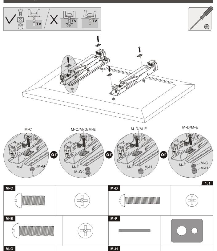
Note: Choose the appropriate screws, washers and spacers (if necessary) according to the type of screen. • Position the adapter brackets as close as possible to the center of the display. - Screw the adapter brackets onto the display.
