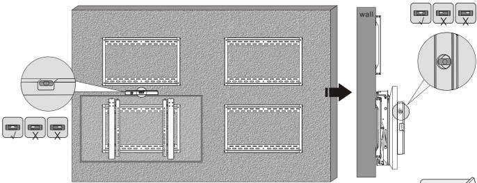
Adjust the display to keep level in vertical and horizontal directions.
