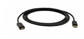
Kramer's C-DPM/HM/UHD enables you to connect your DisplayPort<sup>™</sup> equipped PC or laptop to an HDMI display with no additional adapters or cables required. This active DisplayPort to HDMI cable is used for true conversion when the source does not support DP++ and can be used in either DisplayPort single-mode or dual-mode outputs. C-DPM/HM/UHD supports up to 4K@60Hz (4:4:4)
