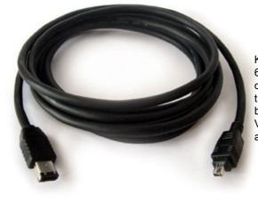
Kramer's C-FM6/FM4 is a high-performance cable with 6-pin FireWire® connectors at one end, and a 4-pin connector at the other. It is used primarily for data transfer (IEEE 1394) at speeds of up to 400Mbps between multimedia devices such as digital cameras, VCRs, CD drives, hard disks, scanners, graphic cards and editing systems
