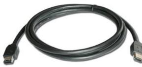
Kramer's C-FM6/FM6 is a high-performance cable with 6-pin FireWire® connectors at both ends. It is used primarily for data transfer (IEEE 1394) at speeds of up to 400Mbps between multimedia devices such as digital cameras, VCRs, CD drives, hard disks, scanners, graphic cards and editing systems
