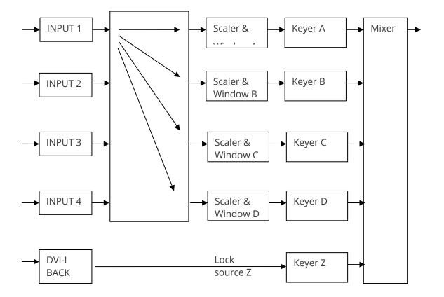
As the diagram shows, the 4 DVI-I inputs are available for use by any of the scalers. A 5<sup>th</sup> DVI-I input acts as a 'lock source' (also known as window Z), which can be used for background / cascading.
