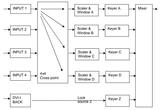
As the diagram shows, the 4 inputs are available for use by any of the scalers. A  $5^{\text{th}}$  DVI-I input acts as a 'lock source' (also known as window Z), which can be used for background / cascading.
