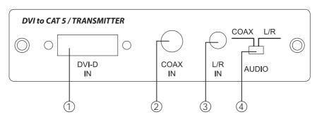
DVI-D IN – Plug from DVI/HDMI source equipment's video output with DVI in cable.
