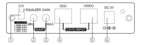
CTI dip switch – Setting CTI by using the twin jumpers to adjust the optimized setting for different distance of connection.
