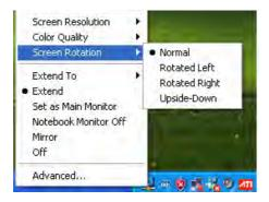
**Extend to:** Reposition the extended screen to the top, bottom, left or right of the primary display.
