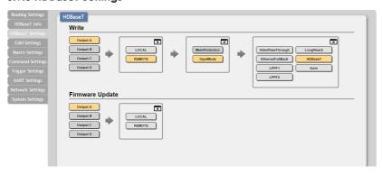
Click on the "HDBaseT Settings" tab to enable or disable various HDBaseT feature support options. This tab also allows you to update the HDBaseT chipset firmware on the transmitter or receiver side.
