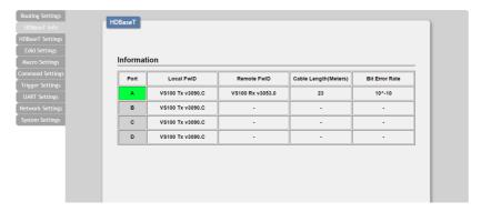
Click on the "HDBaseT Info" tab to view the HDBaseT connection diagnostic information including the current transmitter/receiver firmware versions, measured cable length estimate and current bit error rate.
