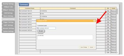
Click on the "Command Settings" tab to create, edit or delete commands. The number of commands that can be stored in the unit is limited by memory. It is generally recommended that commands be under 128 characters long (including spaces). However, if longer commands are needed there is limited support for commands up to 512 characters long. In this case the number of (up to) 512 character commands is limited to 32 and the remaining 96 commands must be under 128 characters.
