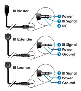
Note: Due to the similarity of the IR Extender and IR Learner cables a part no. "CBL-IR10C3SA200A" sticker has been placed on the IR Learner to help differentiate it.
