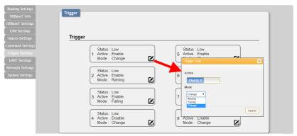
Click on the "Trigger Settings" tab to view the current trigger status and edit trigger behavior. Each trigger has 3 indicators: Status, Active, and Mode.
