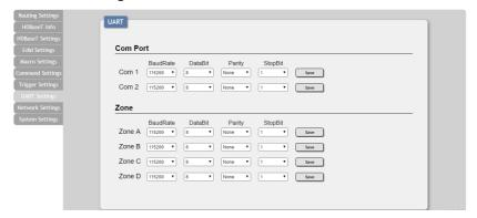
Click on the "UART Settings" tab to configure each COM port's Baud Rate, Data Bit, Parity, and Stop Bit. Values that can't be directly selected here may be set via Telnet or RS-232. After changing a COM port's settings please click on the "Save" button to store the new settings.
