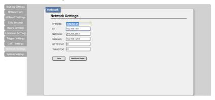
Click on the "Network Settings" tab to change the network settings for the unit. You can manually set the IP address, netmask, and gateway address in "Static IP" mode, or you can obtain an IP address automatically by enabling DHCP. You may also change the default HTTP and Telnet ports used by the unit here. Click on the "Save" button to save your updated network settings.
