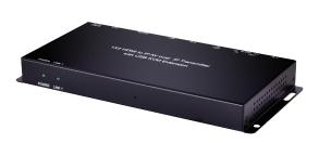
The Dual over IP solution is designed to control and switch between KVM, PCs/ laptops and monitors to any connected devices to controlled dual monitor cross-transmit with single pair of KVM.
