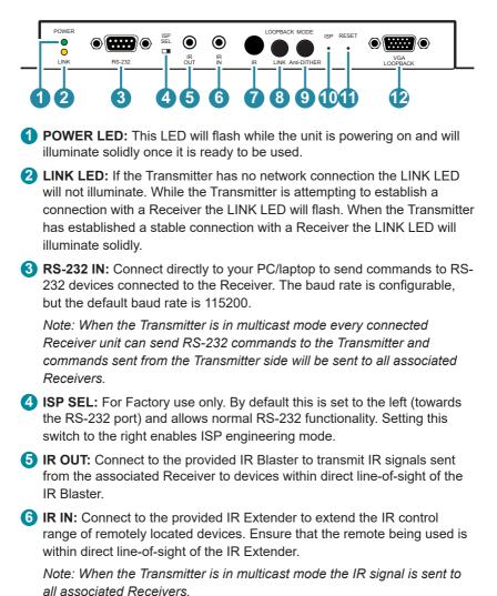
**IR WINDOW:** Accepts IR signals from any standard remote control and sends the signal to the IR Out on the associated Receiver.
