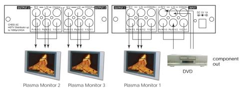
2. Works as a 1-in 3-out distribution amplifier for HD RGBHV video source.
