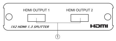
(1) HDMI output 1 to 2: Connect each of the output ports to the HDMI display. When more than one output connected, the HDMI outputs play identical video signal simultaneously.
