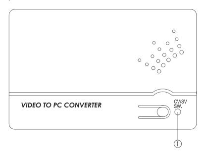
① CV/SV SW & LED: Press this button to switch the input source between composite or S-Video. The LED will turn yellow when switched to composite input and will switch to red when changed to S-Video input.
