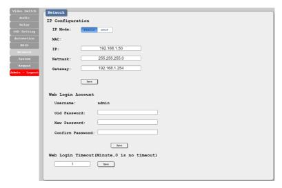
1) IP Configuration: IP Mode may be switched between Static IP or DHCP. In Static IP Mode the IP, netmask and gateway addresses must be manually set. When in DHCP Mode, the unit will attempt to connect to a local DHCP server and obtain IP, netmask and gateway addresses automatically. Please press "Save" after making any changes to the IP configuration or mode.
