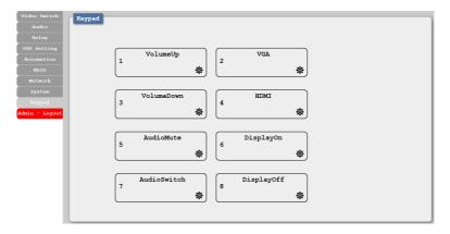
1) Keypad Button Assignment: Click the "Edit" icon (秦) inside each numbered button to assign a unit function or behavior to that button. If the selected function requires additional parameters those can also be configured within the same popup window.
