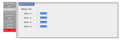
Relay Out Port 1~4: Manually open or close relays 1~4. Selecting "ON" closes the relay, selecting "OFF" opens it.
