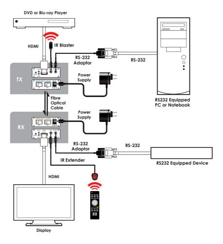
Note: The RS-232 design here works in 2 ways and therefore, no Input/Output determination.
