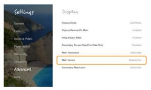
According to your monitor capabilities, set to the maximum supported resolution. If 2 monitors are connected to the unit, the display mode is automatically changed to dual mode and you can set both monitors' resolutions.
