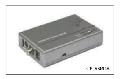
CP-VSRGB is designed for converting Composite video/ S-Video signal such as iPod, DVD, X-Box to the component or RGsB for connecting to SDTV or projector.
