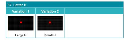
The **Letter H** pattern is a screen filled with a series of large or small capital "H" characters moving vertically up the screen. This is a basic test to confirm motion detail. There are 2 variations: Large "H" characters and small "H" characters.
