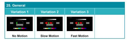
The **General** pattern is an all-purpose, multi-pattern test to visually check for multiple issues simultaneously. It includes color bars, 8-step greyscale, vertical and horizontal multi-burst, cross hatch, circle and an optional motion pattern. There are 3 variations: No motion, slow motion and fast motion.
