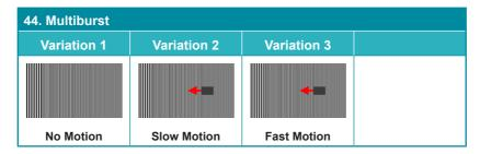
The **Multiburst** pattern provides a standard multiburst pattern consisting of vertical white lines that decrease in thickness from left to right allowing the user to analyze the bandwidth and frequency response of the video path and connected display. There are 3 variations: Standard multiburst, multiburst with a slow moving gray block, and multiburst with a fast moving gray block.
