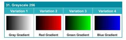
The **Grayscale 256** pattern provides a way to fine tune the contrast, brightness and grayscale tracking of your display with a full 265 step gradient progressing from 0% to 100% brightness. When testing a display, no color should be visible at any point across the gradient, and the transition from black to white should appear even and consistent. There are 3 variations: 256 vertical bars, two sets of 256 vertical bars with the lower set reversed, and 265 horizontal bars.
