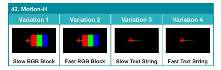
The **Motion-H** patterns are a collection of horizontal motion tests. These can be used to test your display's pixel on/off response time. There are 4 variations: Slow red/green/blue block, fast red/green/blue, slow moving sample text, fast moving sample text.
