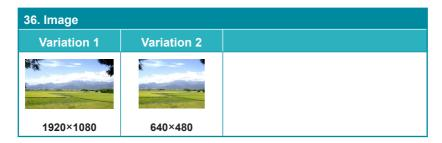
The **Image** pattern is a user customizable test pattern that holds two bitmap images. One image is for use with low output resolutions (below 1920×1080) and the other is for high output resolutions (1920×1080 and above). The low resolution image is a 640×480 bitmap (RGB, 24-bit) and the high resolution image is a 1920×1080 bitmap (RGB, 24-bit).
