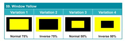
These **Window** patterns are additional screen purity tests offering seven different patterns with different sized windows of each color on a black field: **Blue, Cyan, Green, Magenta, Red, White, Yellow.** The color patterns should display an even distribution of brightness and consistent color tone across the screen. Each pattern has 4 variations: Normal 75% Window, Inverse 75% Window, Normal 50% Window, and Inverse 50% Window.
