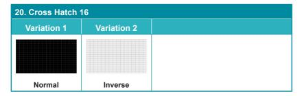
The **Cross Hatch 16** pattern is a full field black & white pattern of crossing vertical and horizontal lines dividing the screen into 16 sections in each direction. This pattern is primarily used to check for color convergence and pincushion issues in projectors. There are 2 variations: Normal (white lines, black field) and Inverse (black lines, white field).
