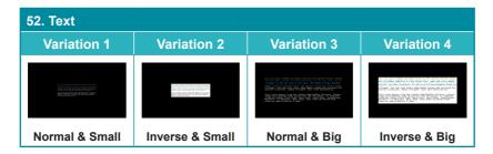
The **Text** pattern is used to check the clarity of text at various sizes and colors. This is primarily a test for projectors. There are 4 variations: Small multi-color text on a black background, small multi-color text on a white background, large multi-color text on a black background, and large multi-color text on a white background.
