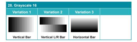
The **Grayscale 16** pattern provides a way to check and adjust the contrast, brightness and grayscale tracking of your display with 16 bars progressing from 0% to 100% brightness in even steps. When testing a display, no color should be visible in any of the bars, and all bars should be visible and distinct. There are 3 variations: 16 vertical bars, two sets of 16 vertical bars with the lower set reversed, and 16 horizontal bars.
