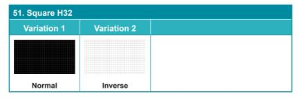
The **Square H32** pattern is a full field black & white pattern of squares dividing the screen horizontally into 32 sections. This pattern is primarily used to check projector linearity. There are 2 variations: Normal (white lines, black field) and Inverse (black lines, white field).
