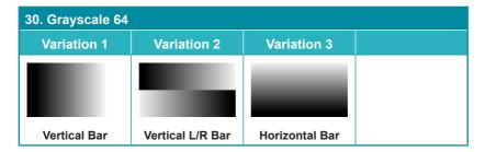
The **Grayscale 64** pattern provides a way to check and adjust the contrast, brightness and grayscale tracking of your display with 64 bars progressing from 0% to 100% brightness in even steps. When testing a display, no color should be visible in any of the bars, and all bars should be visible and distinct. There are 3 variations: 64 vertical bars, two sets of 64 vertical bars with the lower set reversed, and 64 horizontal bars.
