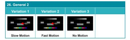
The **General 2** pattern is a simplified all-purpose, multi-pattern test to visually check for multiple issues simultaneously. It includes color bars, 8-step greyscale, vertical and horizontal multi-burst, multi-color center/edge alignment lines, and an optional block motion pattern. There are 3 variations: No motion block, slow motion and fast motion.
