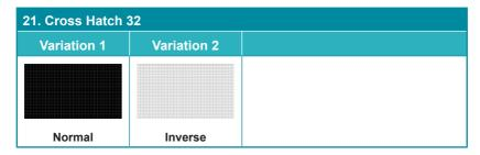
The **Cross Hatch 32** pattern is a full field black & white pattern of crossing vertical and horizontal lines dividing the screen into 32 sections in each direction. This pattern is primarily used to check for color convergence and pincushion issues in projectors. There are 2 variations: Normal (white lines, black field) and Inverse (black lines, white field).
