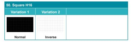
The **Square H16** pattern is a full field black & white pattern of squares dividing the screen horizontally into 16 sections. This pattern is primarily used to check projector linearity. There are 2 variations: Normal (white lines, black field) and Inverse (black lines, white field).
