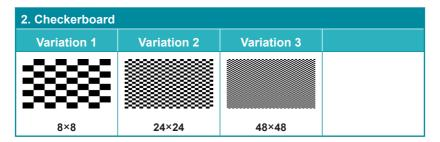
The **Checkerboard** pattern displays a repeating black and white checkerboard image. This is ideal for checking the alignment and corner convergence of TVs or monitors. Bandwidth can be checked by observing the vertical transitions. Transitions from black to white should be sharp. There are 3 variations: 8×8, 24×24 and 48×48.
