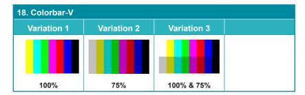
The **Colorbar-V** pattern comes in 3 variations. The first is a standard (white, yellow, cyan, green, magenta, red, blue, black) 100% color bar pattern using vertical bars. The 2nd variation has all bars at 75% brightness. The 3rd variation is split with the top half being at 100% and the lower half being at 75% brightness.
