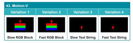
The **Motion-V** patterns are a collection of vertical motion tests. These can be used to test your display's pixel on/off response time. There are 4 variations: Slow red/green/blue block, fast red/green/blue, slow moving sample text, fast moving sample text.
