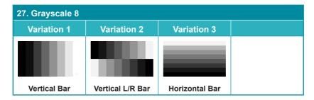
The **Grayscale 8** pattern provides a way to check and adjust the contrast, brightness and grayscale tracking of your display with 8 bars progressing from 0% to 100% brightness in even steps. When testing a display, no color should be visible in any of the bars, and all bars should be visible and distinct. There are 3 variations: 8 vertical bars, two sets of 8 vertical bars with the lower set reversed, and 8 horizontal bars.
