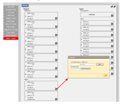
The two HDMI outputs (port I & port J) allow support for the maximum HDMI timing up to 6G (4096×2160@60Hz) and can be used for normal source routing (listed as "Independent" within the WebGUI) and mirroring (listed as "Mirror" within the WebGUI) for local monitoring purposes or zone monitoring (e.g. The HDBaseT output connects to a TV in a remote zone the local HDMI connection goes into an AVR).
