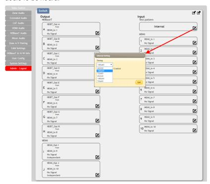
Timing: Test patterns can be generated with the following standard timings: 720p@50/60Hz, 1080p@50/60Hz, 4K@25/30Hz. Test pattern output does not use HDCP.
