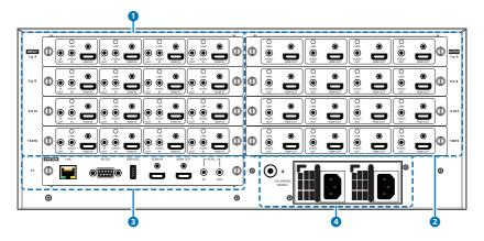
INPUT 1 ~ 16 Card Slots: These four high bandwidth card slots accept a variety of specially designed video input cards. Each card typically has 4 primary inputs along with additional auxiliary I/ O ports as needed.
