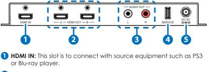
2 HDMI OUT: These slots are to connect with UHD display/TV for images display. Each output can be displaying with different timing and pattern and image.
