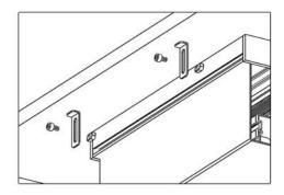
3. Place the L tighteners onto the fixing points.
