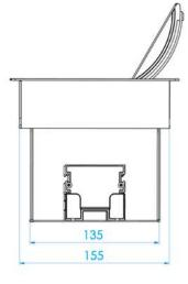
Link Power Module, 1xUK Socket, 1xSC: 203mm
